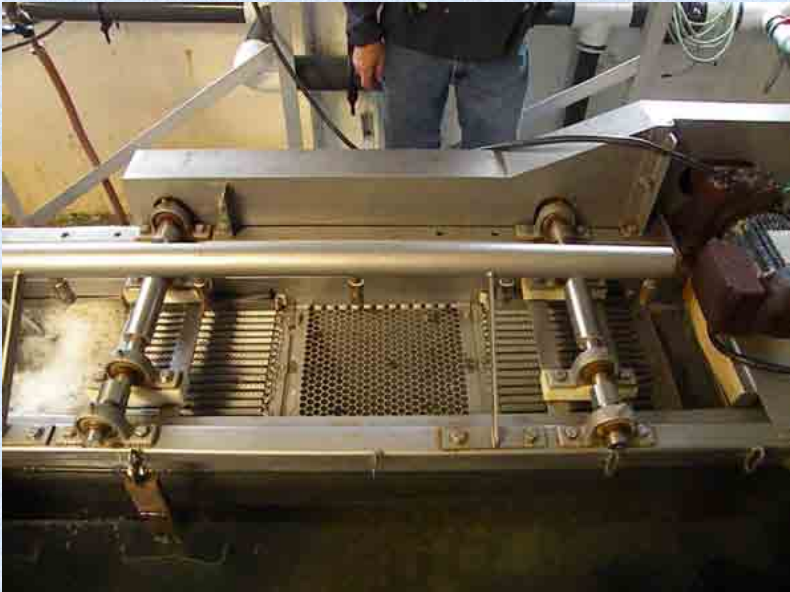
Scallop seed grader, rotates in and out of a water bath. Scallops pass through parallel spaces, mussels and other shellfish pass through holes. Several panels, with increasing space and aperture sizes.
