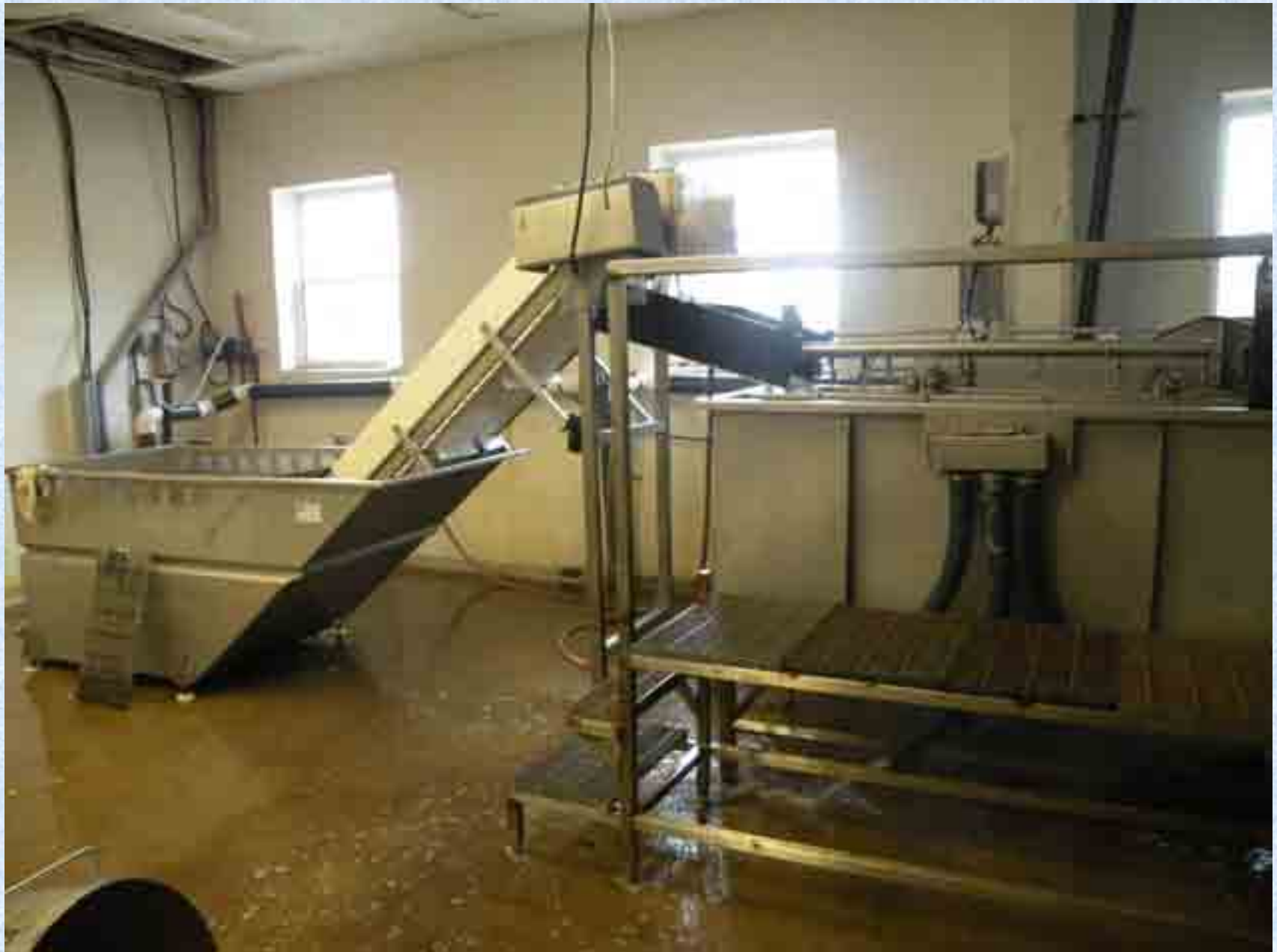
Processing line for sorting/grading scallop spat from bags. Hopper (L), conveyer, grader.
