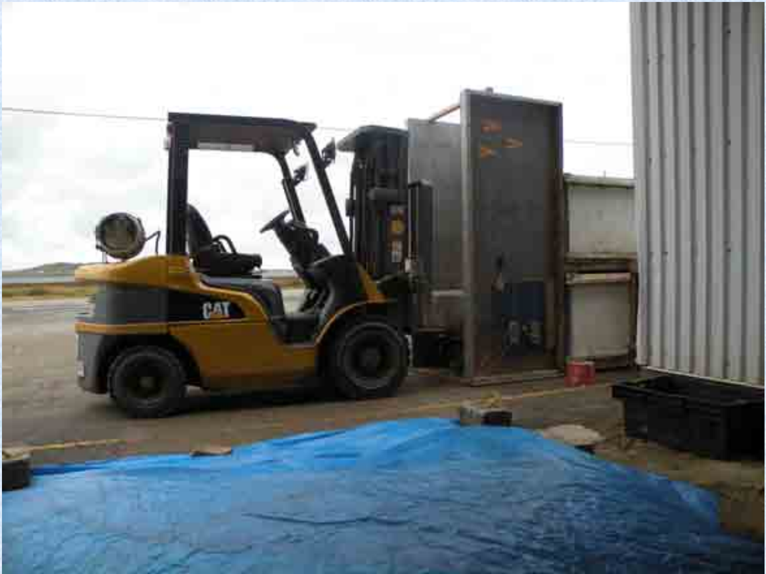
Lines of spat bags are assembled, then put into the form on the right; a big concrete block lowered on to them, then tied in a bundle to save room on the vessel.
